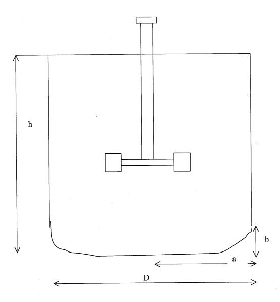
The above diagram represents the batch reactor.
