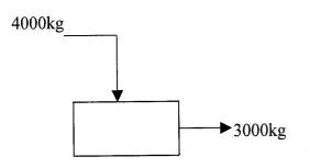
The starting raw material (plantain pod) is reduced into ashes. The starting material is 4000kg (0.4T) of plantain pod, which is reduced to 3000kg (0.03T) of ashes. From lab work 400g of plantain pod is reduced to 300g therefore the scale-up factor is
