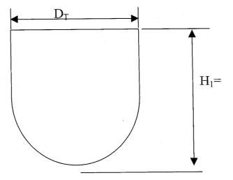
Note that Height of Cylindrical part = Diameter of Extractor
