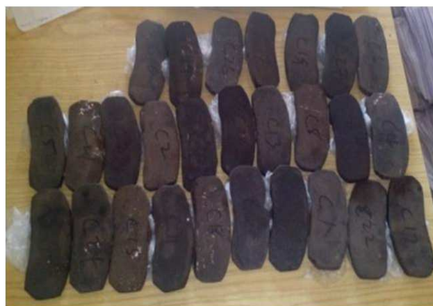
Fig. 1: Heat treated Friction Lining Samples
