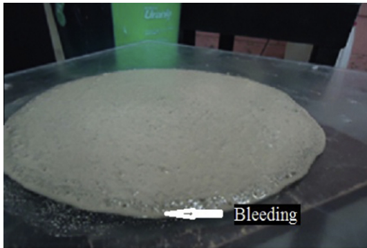
Fig. 9. Flow spread of mortar with bleeding (30M1, 2.0% HRWR).
