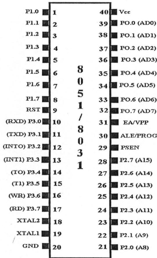
Fig.3.10 AT8952 Pin Function
