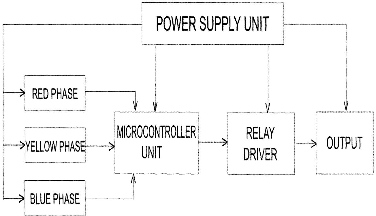
Fig 3.1 Block diagram of automatic 3 phase change over and Generator starter/stopper.
