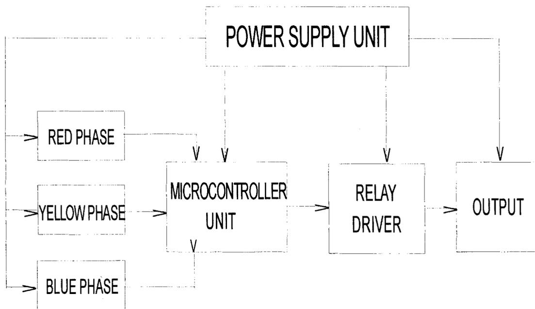
Fig 1.1 Block diagram of automatic three phase change-over and generator starter
