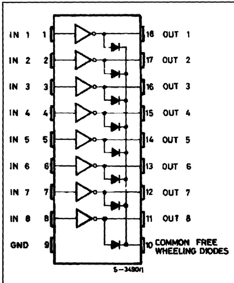
Fig3.6 Pin connection of UNL2803.
