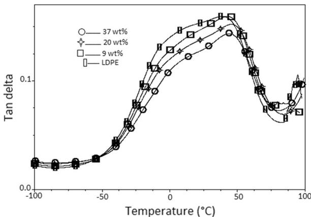
**Fig. 6** Variation of  $\tan\delta$  with temperature in LDPE and untreated wood composites at different filler loading
