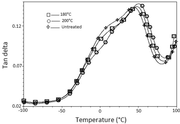
**Fig. 7** Dependence of  $\tan\delta$  on temperature for composites made from 37 wt% untreated and heat treated wood flour
