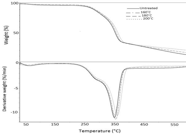
Fig. 1 TGA/DTG thermograms of untreated and heat-treated wood flour
