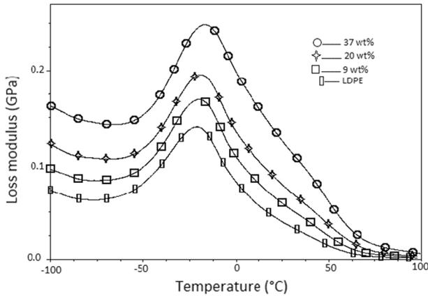
**Fig. 4** Loss modulus curves of composites made from untreated wood flour at different filler loading
