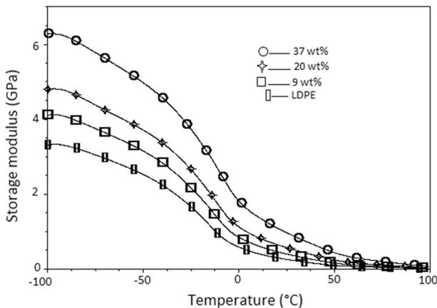
Fig. 2 Storage modulus of LDPE and composites as a function of wood content
