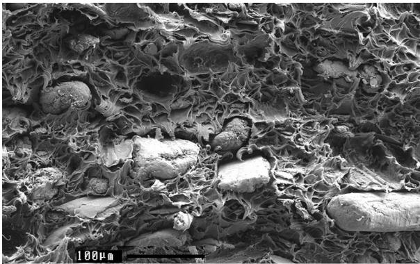
**Fig. 9** Impact fractured surface of untreated wood composites at 37 wt%
