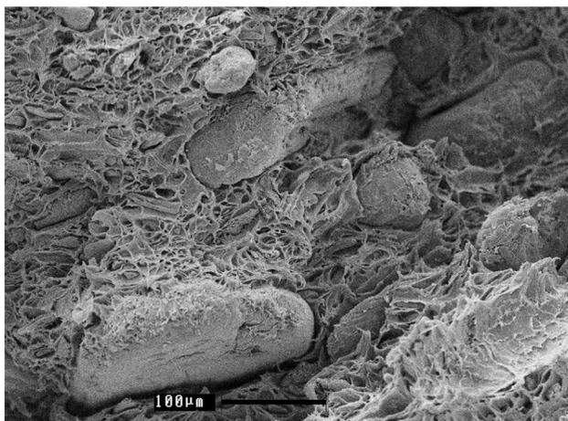
**Fig. 10** Impact fractured surface of composites from wood treated at 200 °C at 37 wt% filler loading showing no sign of ductility
