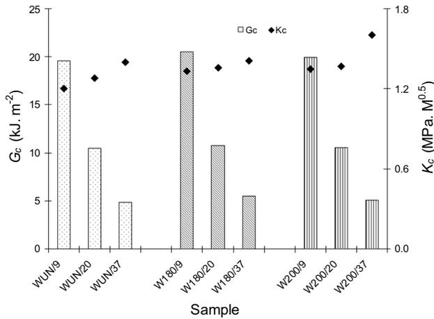
**Fig. 11** Changes in  $K_c$  and  $G_c$  of composites as a function of wood content and treatment temperature
