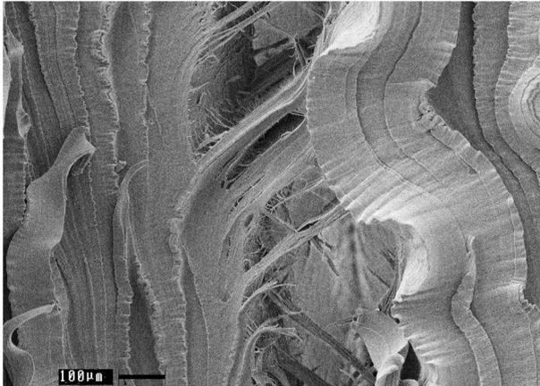
**Fig. 8** Impact fractured surface of neat LDPE showing signs of ductility
