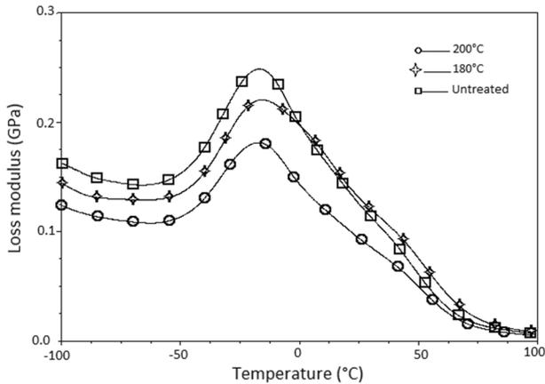
**Fig. 5** Loss modulus curves of composites containing 37 wt% wood flour at different treatment temperature
