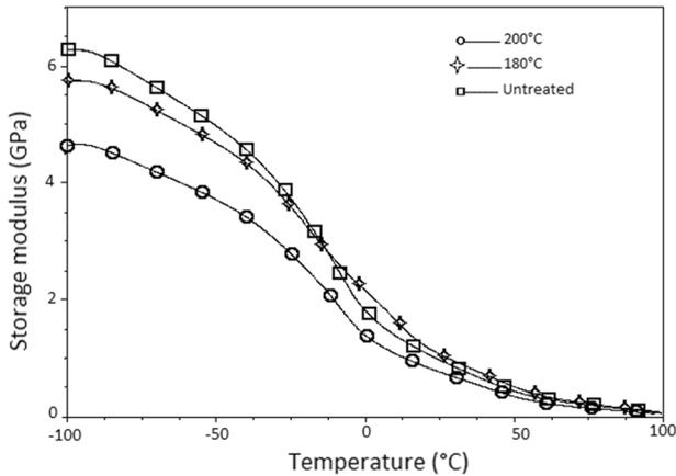
**Fig. 3** Storage modulus of 37 wt% composites as a function of heat treatment
