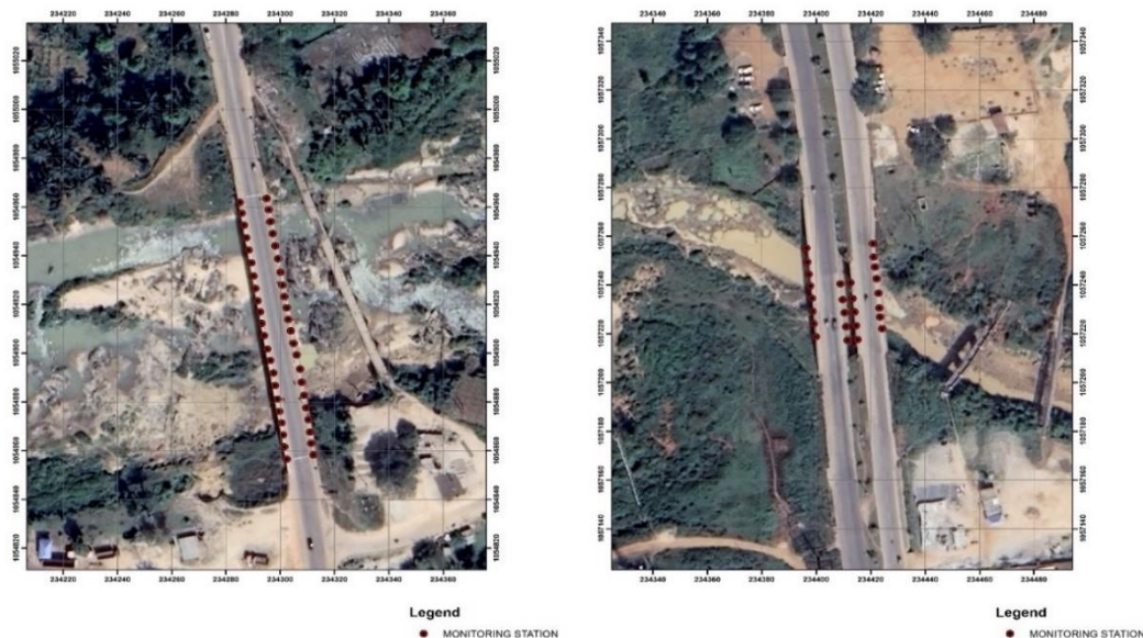
Figure 1: Monitoring stations for bridge A AND B
