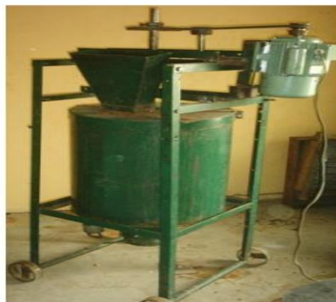
Plate V: Locust Bean Depulping Machine (Source: Olaoye, 2011)
