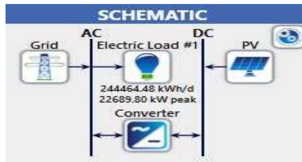
Figure 4.1: Optimal System architecture
