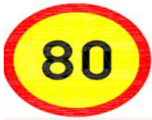
Figure 2. 11: Maximum Speed Limit (Source: Highway Manual Volume VI, 2013)
