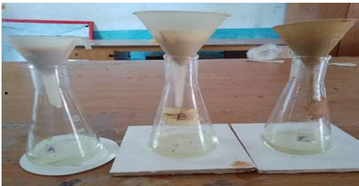
Plate IV: Dealumination of metakaolim
