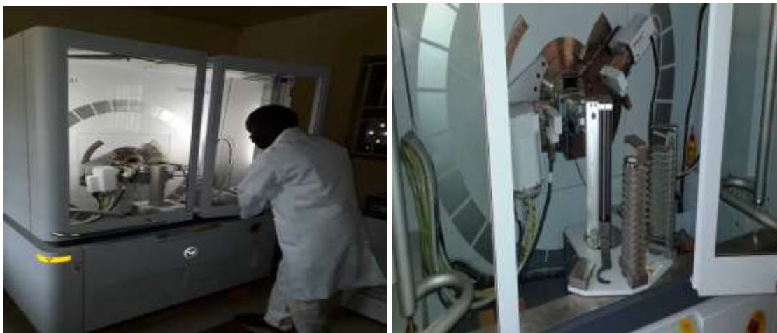
Plate VI: Empyrean Multi-Purpose Research X-ray Diffractometer
