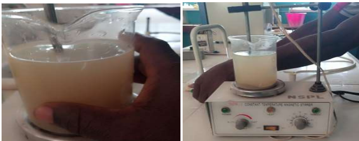
Plate III: Beneficiation of raw Bambu clay
