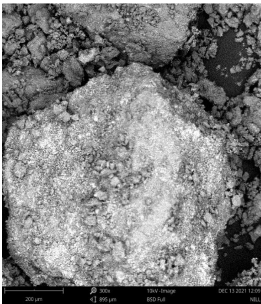
Plate XIV: SEM Image of Synthesized Mg(OH) 2
