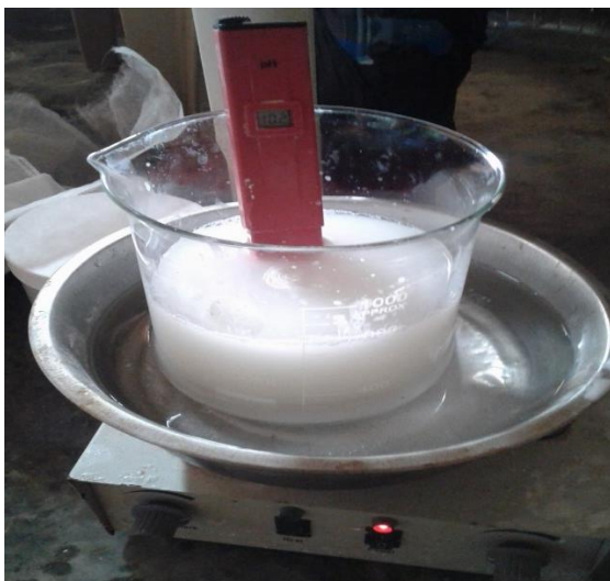
Plate VI: Experimental Setup for the Precipitation of Mg(OH)_2
