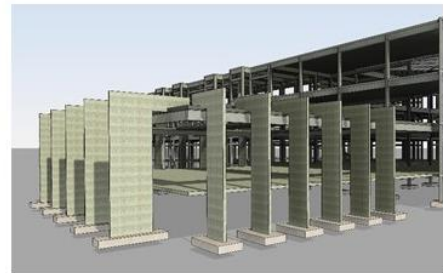
Structural system of the entrance fins
