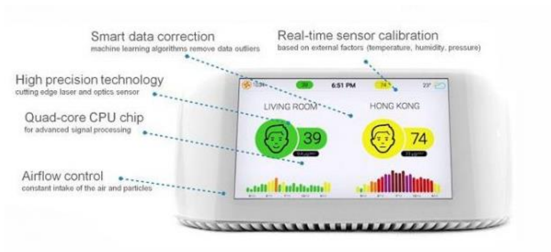
Figure 3.1 Air visual node monitoring device.
