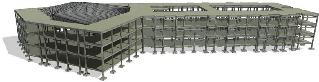
An aerial view showing generally, the monolithic structural system
