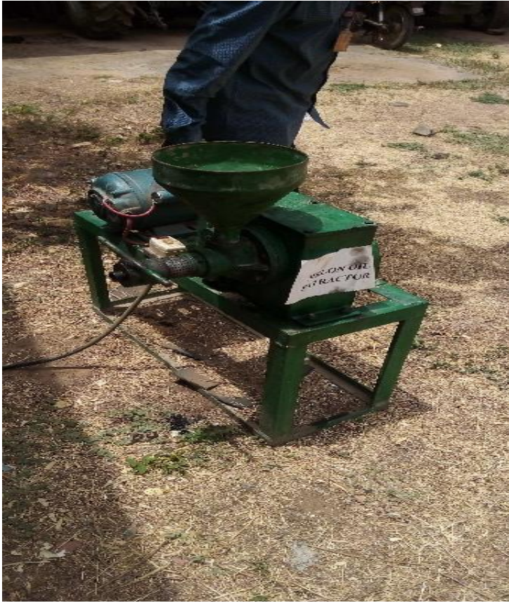
Plate VIII: Locally fabricated oil extractor
