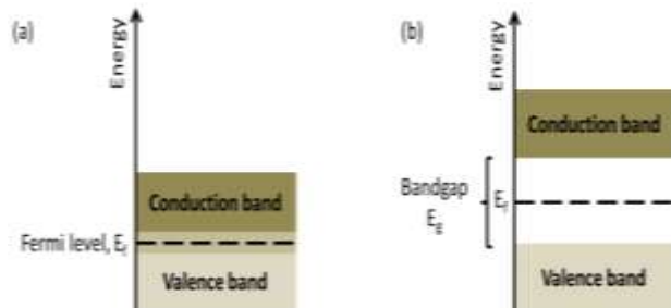
Fig. 4: Energy band gaps and the Fermi level in a (a) metal and (b) pure semiconductor.
