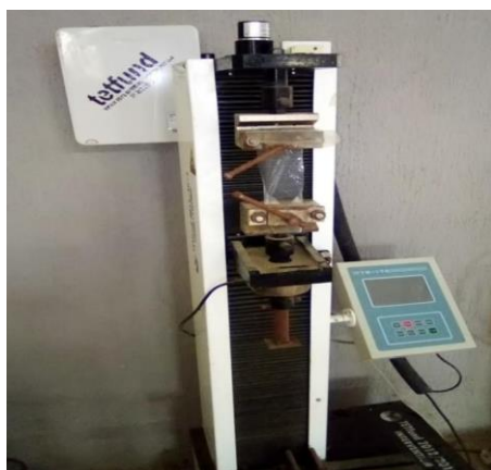
Figure 1: Tensile Strength Machine with Load indicator attached
