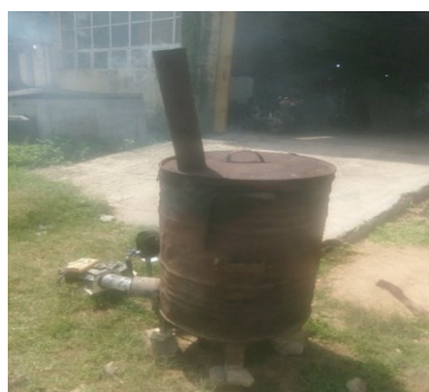
Figure 1: Set-up for ashing of corncob and guinea corn husks using an improvised incinerator
