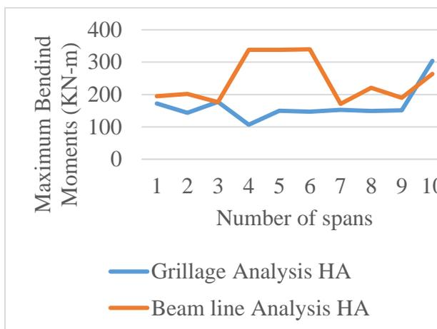
**Fig. 4a:** Bending Moments for Maximum Span Moments for HA loading
