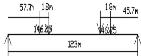
**Fig. 2:** Static Diagram for Maximum Moment and Shear.
