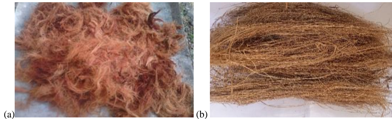
Figure 1: Coir fibre (a) un-treated, (b) treated
