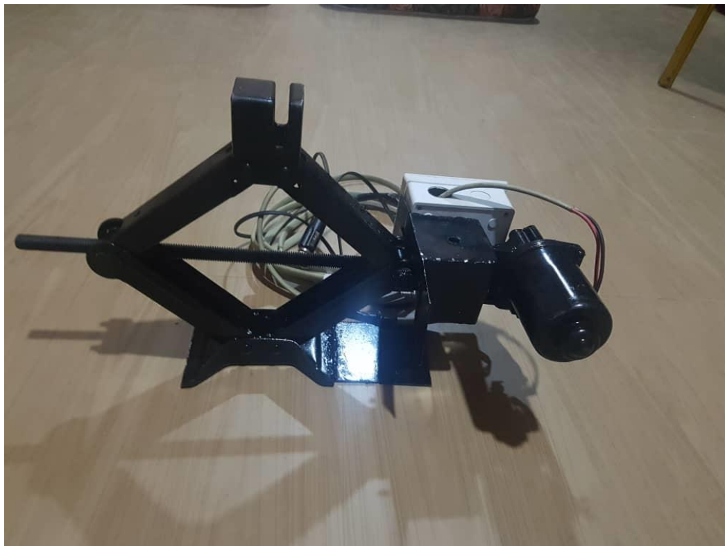
Figure 4 Side view of Android Controlled Automated Scissors car Jack (Source: Duniya and Babatunde, 2021)
