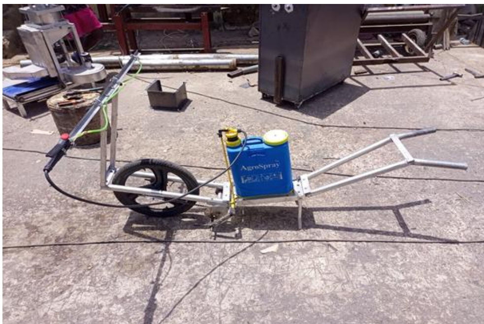
Figure 1: One wheeled, detachable four nozzles sprayer setup
