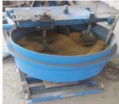
Figure 4: Revolving pan mixer for mixing fibrous concrete
