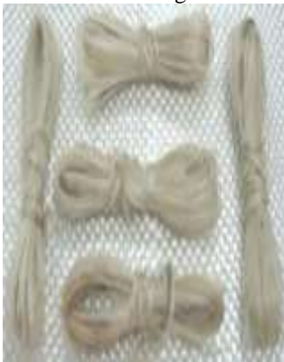
(a) Fibre sample prepared for density test
