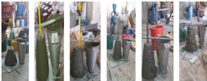
Figure 8: Slump of PC and KBFCC
