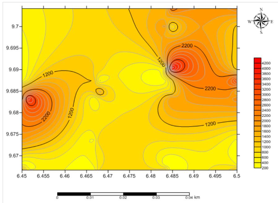
Figure 9: Isoresistivity Map of Vertical Electrical Soundings at 80m of part Maikunkele, Minna, Nigeria
