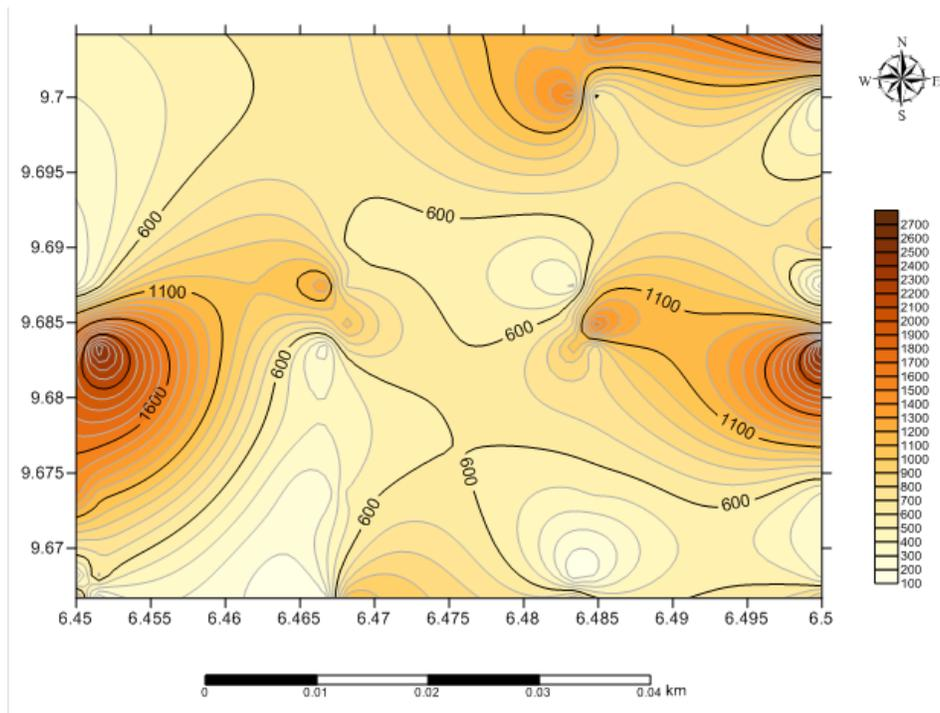
Figure 8: Isoresistivity Map of Vertical Electrical Soundings at 60m of part Maikunkele, Minna, Nigeria
