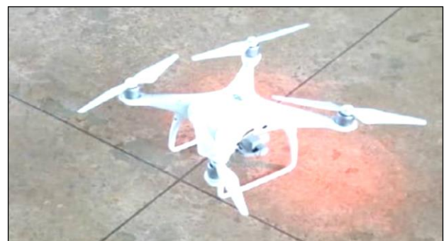
Fig.5: A DJI Phantom 4 Pro Drone used for image data acquisition.
