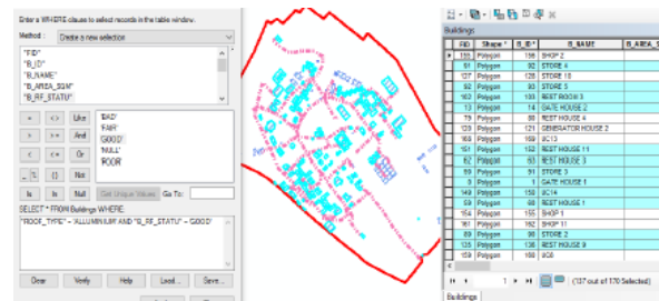
Fig 8: Query Showing building roof type and status Aluminum Roof in Good Condition Syntax= “ROOF_TYPE” = ‘Aluminum’ AND “BRF_STATU” = ‘GOOD’
