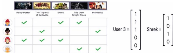
Figure 8. Vector Diagram of Movie to User Synergy
