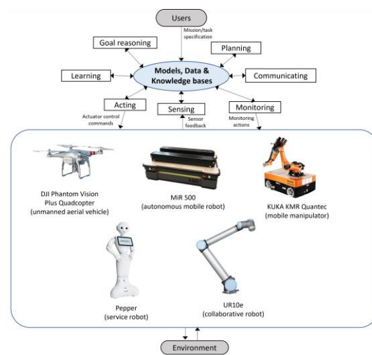
Figure 6. Overview of RAS, including various key functionalities and examples of robots used in manufacturing industry (adapted from [4])
