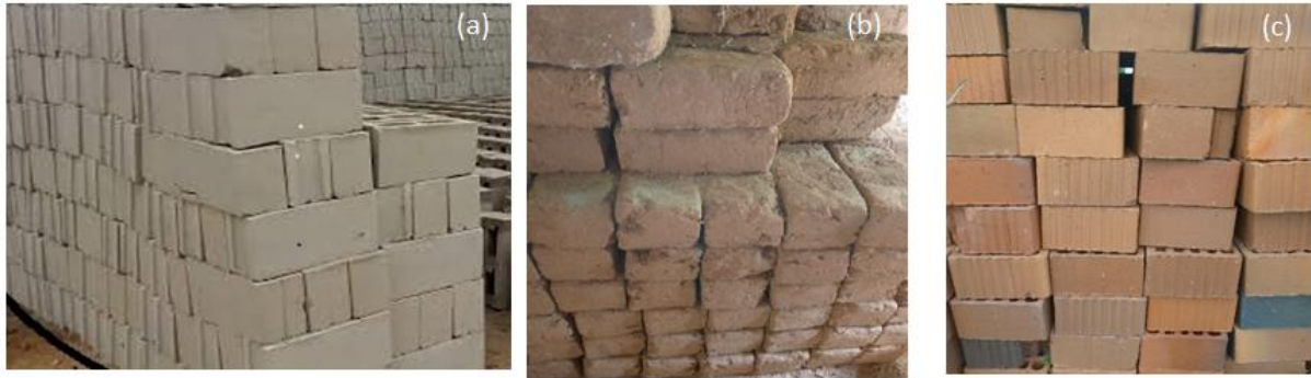
Plate I: (a) Solid concrete Block (b) Mud clay block and (c) Common Solid Burnt clay Bricks
