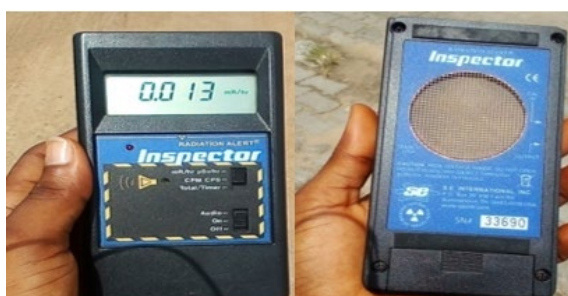
Figure 1: Back and Front view of the Radiation Monitoring Device- Radalert x100
