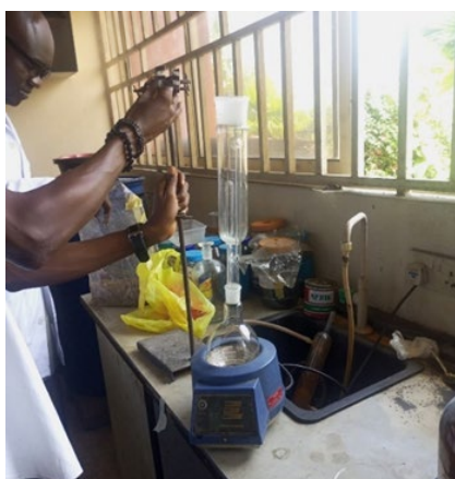
Figure 3: Setting up Soxhlet extraction apparatus
