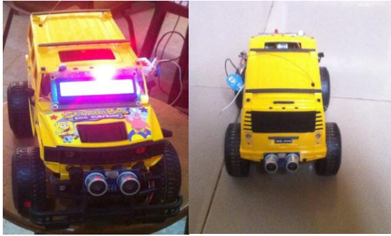
Fig. 6. Front and rear view of the prototype showing ultrasonic sensors
