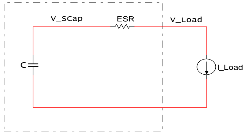
Figure 6. An ideal supercapacitor circuit model
