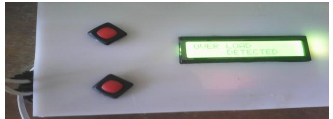
PLATE I: PROJECT CASING AND LCD RESULT SHOWING OVER LOAD DETECTED DUE TO EXCESS CURRENT
