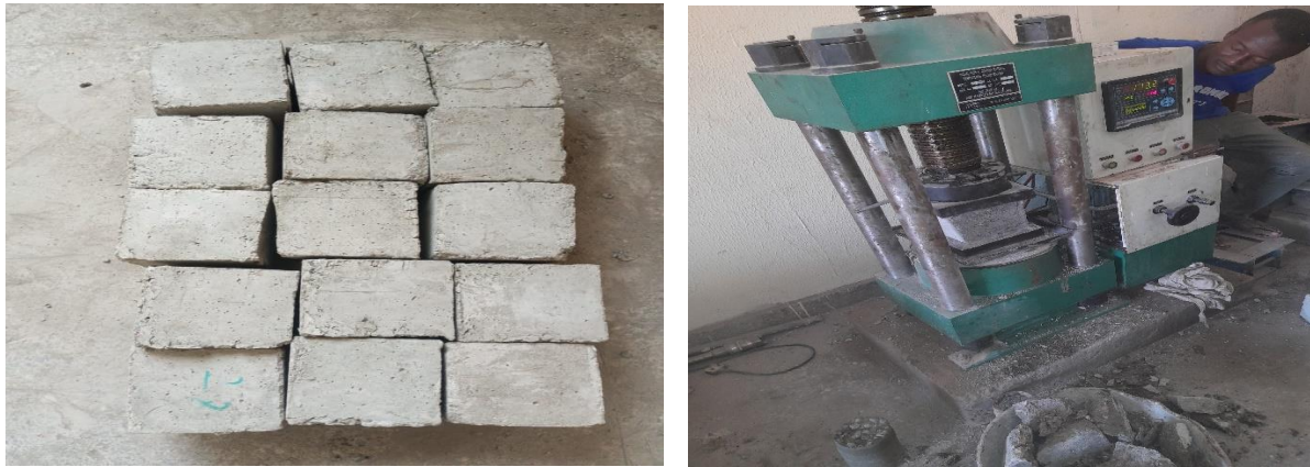
Figure 2: Crushing of cube specimen
