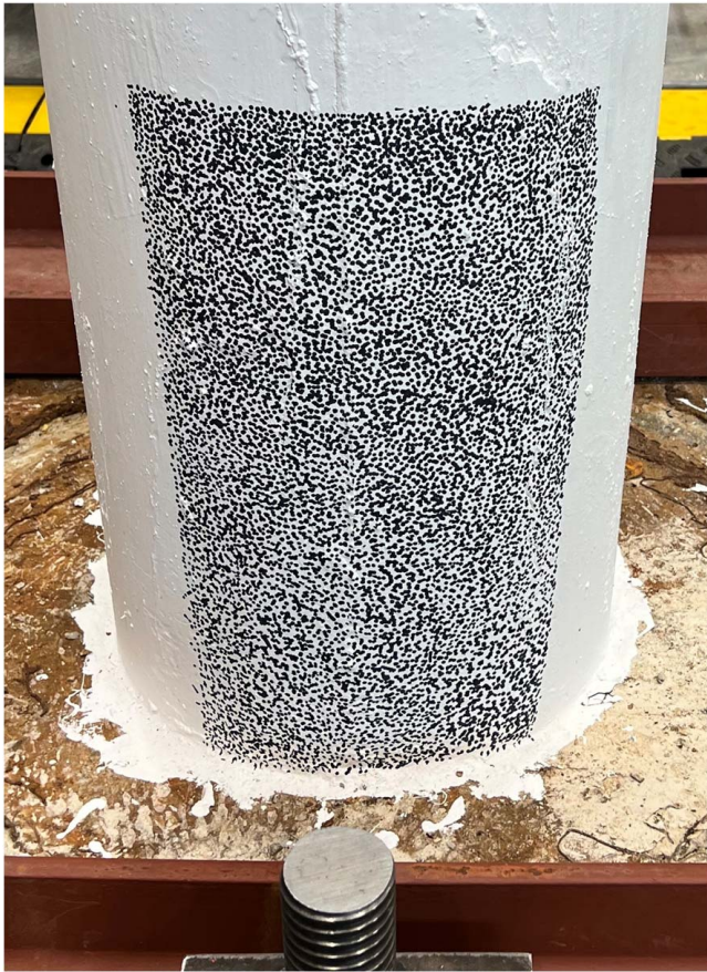
Fig. 6. Speckle pattern for DIC.
