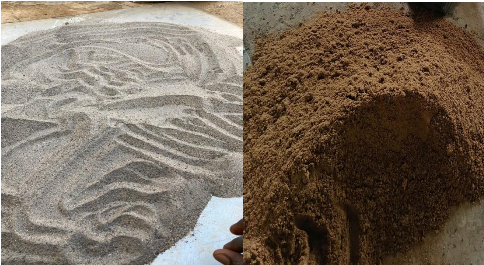
Figure 2. Photographic images of Itakpe Iron ore tailings and Natural Sand
