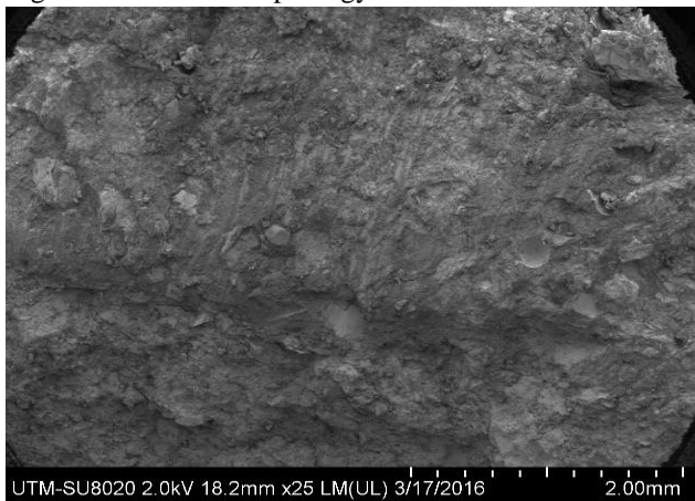
Figure 7: FESEM Morphology of conventional concrete
