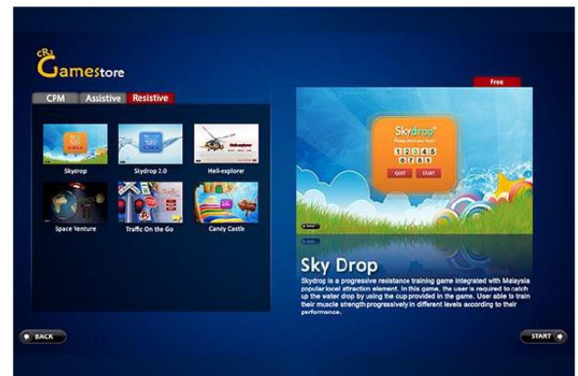
Figure 8: Therapy program control panel, which enables the therapist to customize the therapy based on each patient's requirements. The option includes the training program, range of movement, strength, level of difficulties, repetition and sequence.
