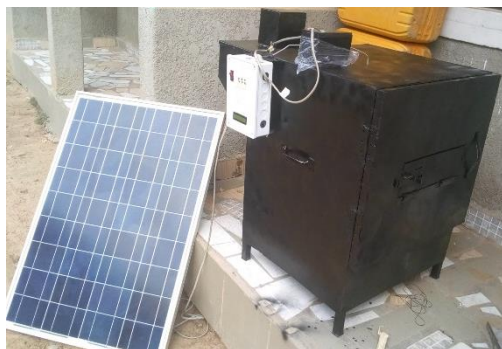
Figure 2: Assembled Solar powered Battery forge
