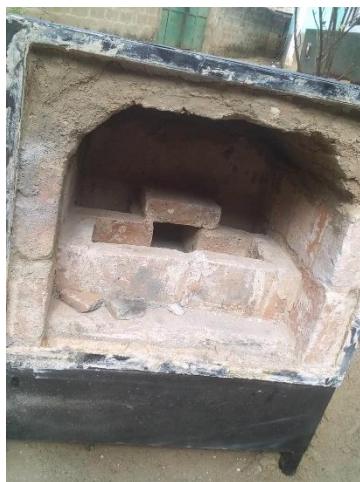
Figure 1: Heating chamber of a Solar powered battery forge
