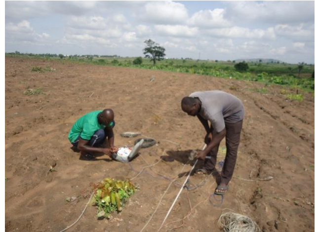
Figure 5: 2D Electrical Resistivity Data acquisition
