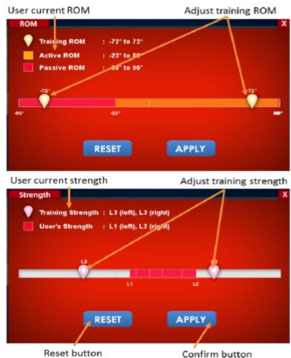
Figure 6: Adjustment panel: Training range adjustment panel (top) and strength adjustment panel (bottom)
