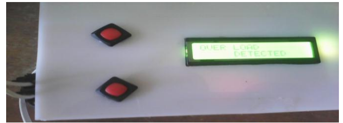
PLATE I: PROJECT CASING AND LCD RESULT SHOWING OVER LOAD DETECTED DUE TO EXCESS CURRENT
