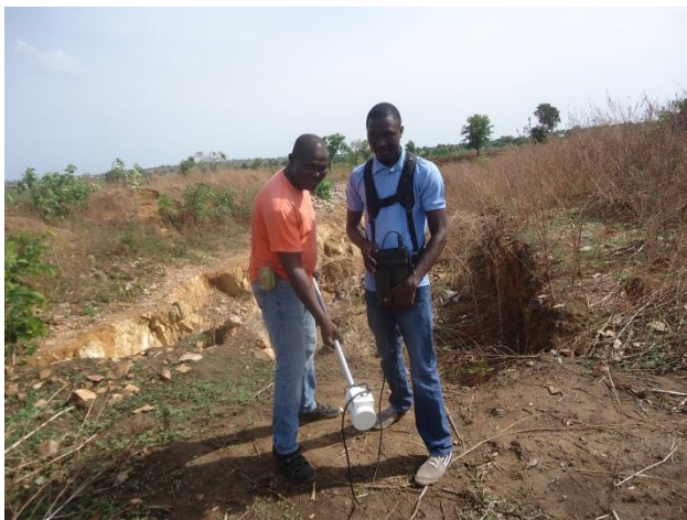
Figure 5: 2D Electrical Resistivity Data acquisition
