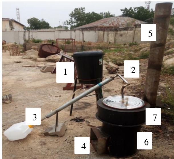
Plate I: The set-up of the water distiller from various parts. Where: 1- Tank for coolant, 2- Condenser, 3- Distillates container, 4- Fuel rack inlet, 5- Chimney, 6- Pot and 7- Stove respectively.
