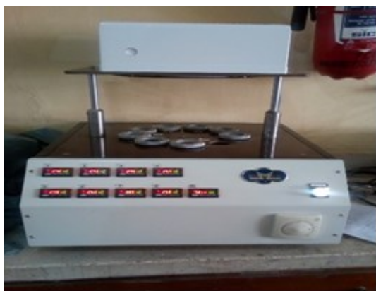
Plate 3.5 Watber vapour Permeability test machine Lastometer Test
