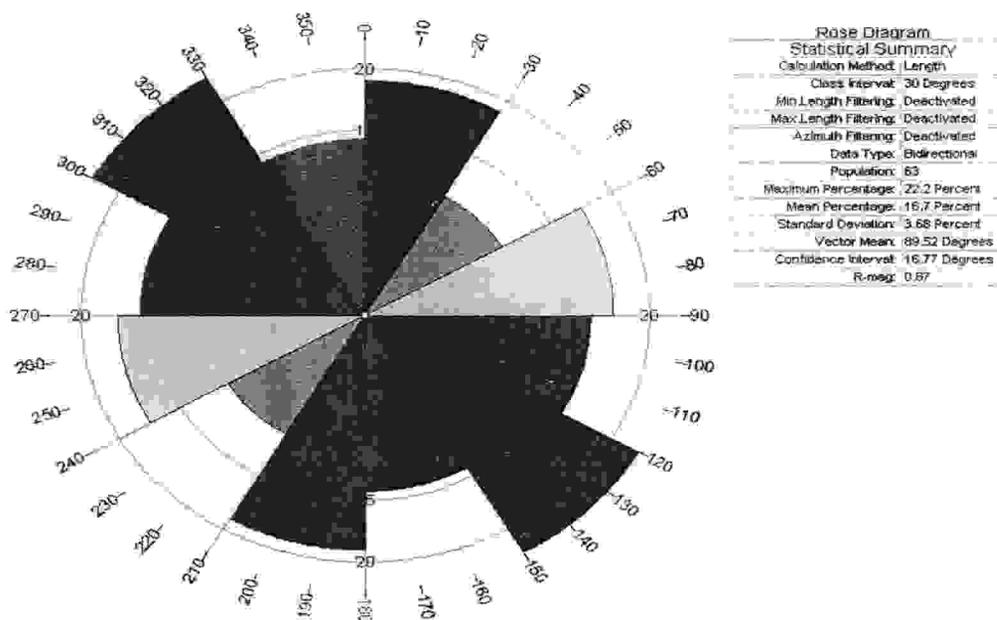
Fig. 7: Rosset diagram showing the principal joint directions
