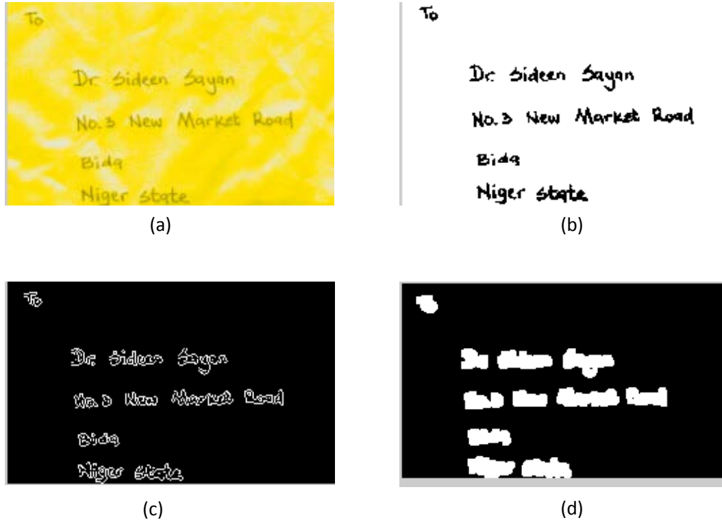
Figure 6: Intermediate stages of processing (a) original address envelop; (b) image segmentation; (c) after edge finding; (d) after binarization and dilation.
