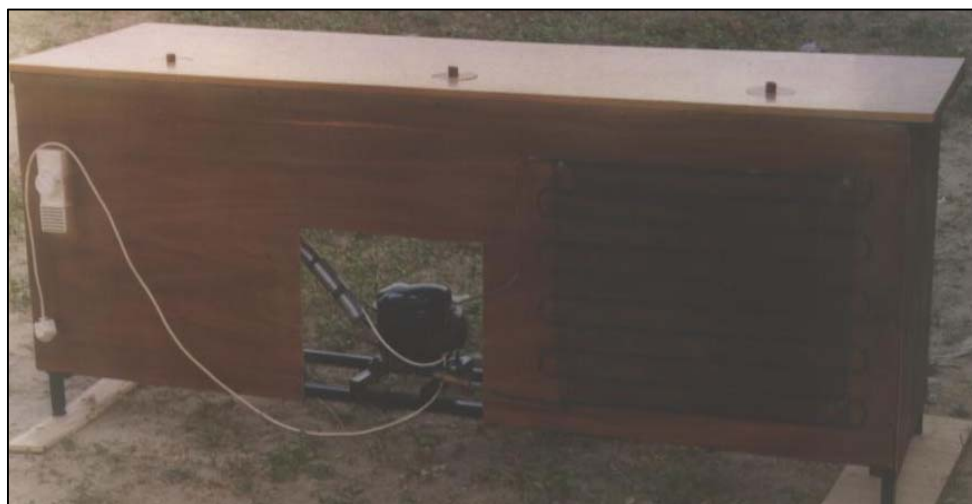
Figure 3. Back view showing condenser, compressor and thermostat of the cooling Table
