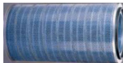
Figure 2. Pulse filters after cleaning
