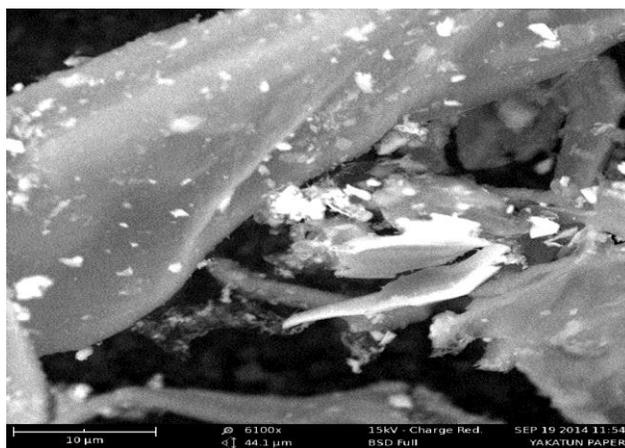
Figure 5: SEM image of the morphological analysis of carbonized paper
