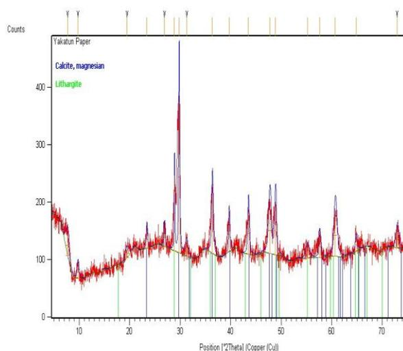
Figure 2: XRD pattern of paper- matching compounds in selected MSW
