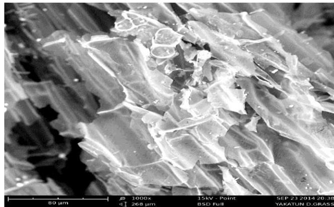
Figure 4: SEM analysis of carbonized dried grass.
