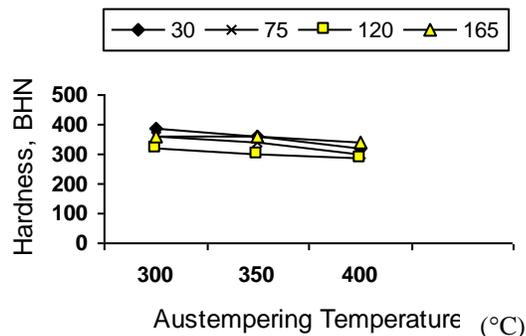
Figure 4: Variation of Hardness with Austempering Temperature for given Austempering Times (30, 75, 120 and 165 mins)
