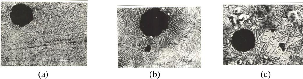
Figure 7: Scanning Electron Micrographs of Ductile Iron Austempered at 300°C for (a) 75 mins (b) 120 mins (c) 165 mins ( $\times 400$ )
