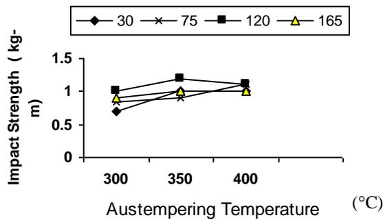
Figure 6: Variation of Impact Strength with Austempering Temperature for given Austempering Times (30, 75, 120 & 165 mins)
