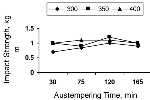
Figure 12: Effect of Austempering Time on Impact Strength for given Austempering Temperatures (300°C, 350°C and 400°C)
