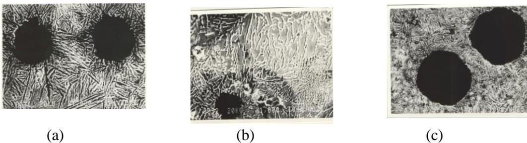
Figure 8: Scanning Electron Micrographs of Ductile Iron Austempered at 350°C for (a) 75 mins (b) 120 mins (c) 165 mins ( $\times 400$ )
