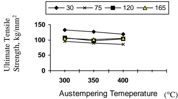
Figure 5: Variation of U.T.S. with Austempering Temperature for given Austempering Times (30, 75, 120 and 165 mins)
