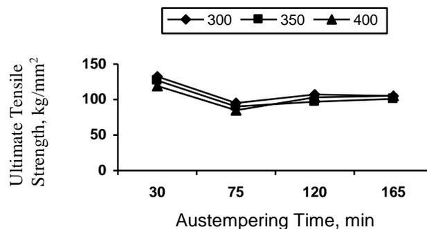
Figure 11: Effect of Austempering Time on U.T.S. for given Austempering Temperatures (300°C, 350°C and 400°C)
