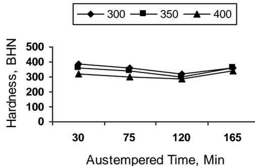
Figure 10: Effect of Austempering Time on Hardness for given Austempering Temperatures (300°C, 350°C and 400°C)
