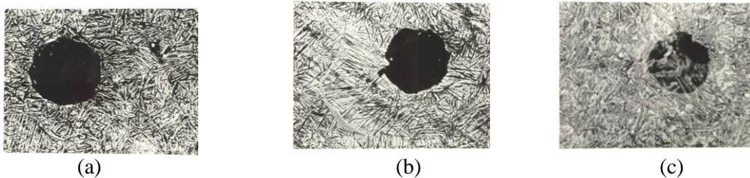
Figure 3: Micrographs of Ductile Iron Austempered at 900°C for 1 ½ hours and Austempered for 30 minutes at (a) 300°C (b) 350°C (c) 400°C ( $\times 400$ )
