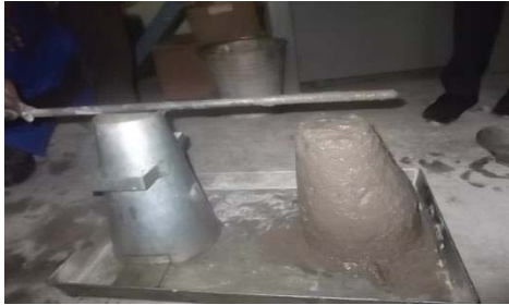
Figure 4. Set up for Slump Test
