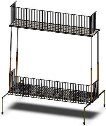
Appendix 10: The highest platform elevated to maximum height
