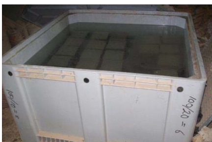
Figure 6. Curing of Concrete Cubes
