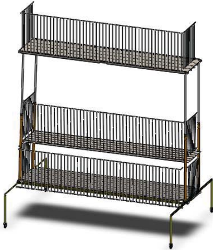
Appendix 11: The middle platform with the safety rails in place
