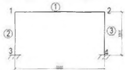
Figure 3(d): The member and joint information
