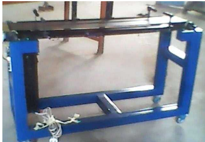
Plate VII. Mini-conveyor after finishing
