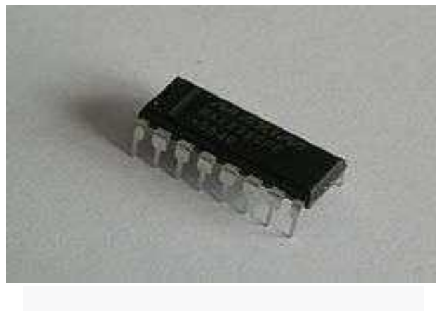
Plate I. MAX232 chip in DIP-16 package (Source: Texas Instrument incorporated, 2014)[14]
