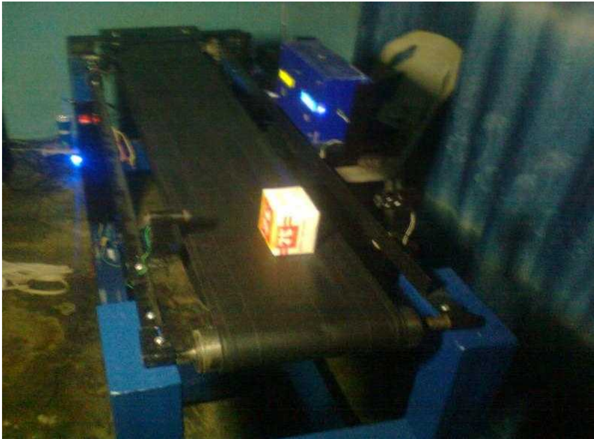
Plate XII. Product between sensors at the exit point
