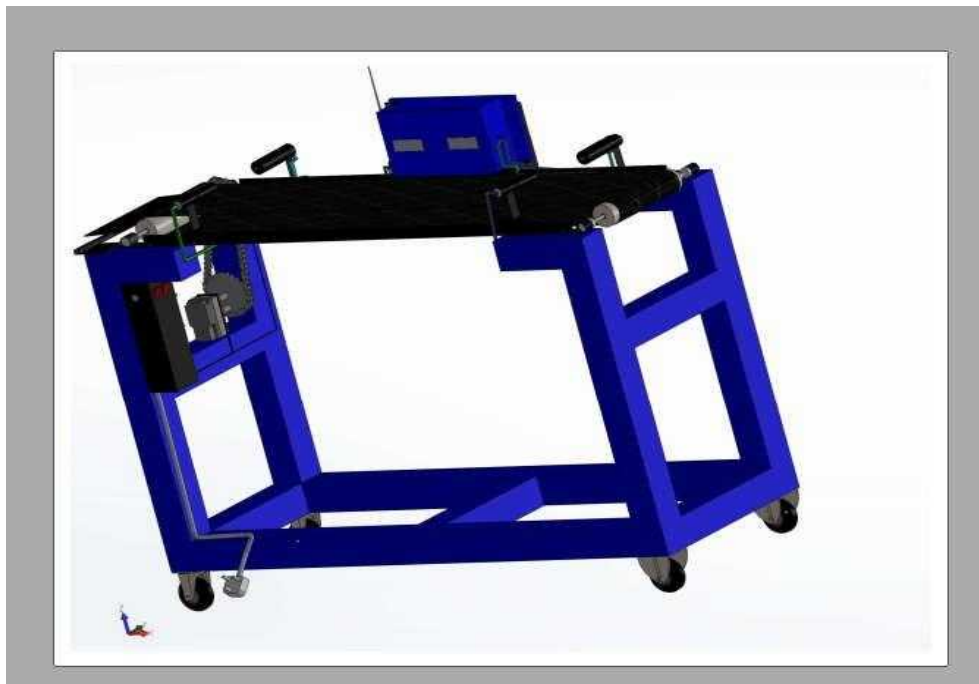
Fig. 19a. 3D Solid work design of mini-automatic conveyor after design calculations and before fabrication
