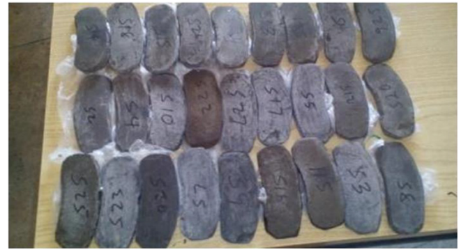
Fig. 2. Heat treated Seashell Reinforced Brake pad Samples.
