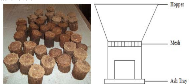
Figure 1: Materials; (a)-Cylindrical briquettes, (b)-Briquette stove
