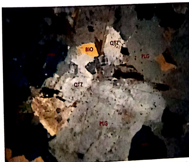
Plate IX: Photomicrograph of granite (Mag.X10)
